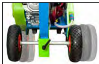
Rear tubeless puncture-proof wheels and adjustable axle.
