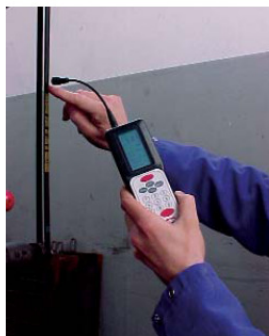
TENSION CONTROL BY VIBRATION METHOD
